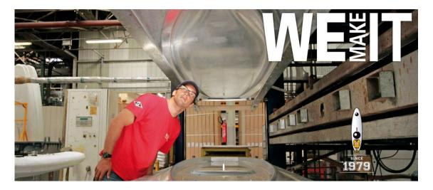
BIC Sport is the proud owner of an industrial tool that is unique in the world, capable of three different manufacturing techniques: thermoforming, thermoforming around a polystyrene core, and blow molding/blown extrusion.
